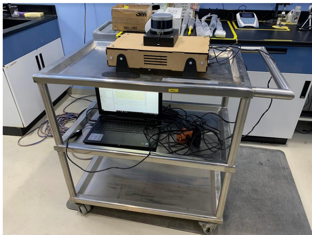
Figure 2. Setup configuration consisting on a Puck Hi-Res and Laptop
